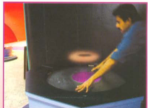
Smoke Ring: The vapour from a humidifier is forced through a circular opening creating perfect smoke rings like a vortex.
